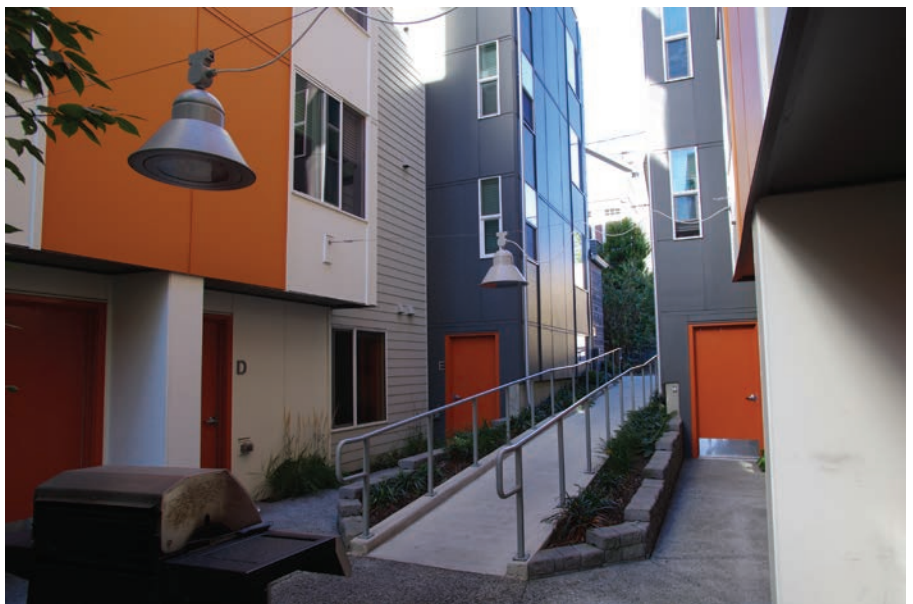
Photo H-4. Accessible townhouses - while individual units have internal staircases, each front door is fully accessible.
